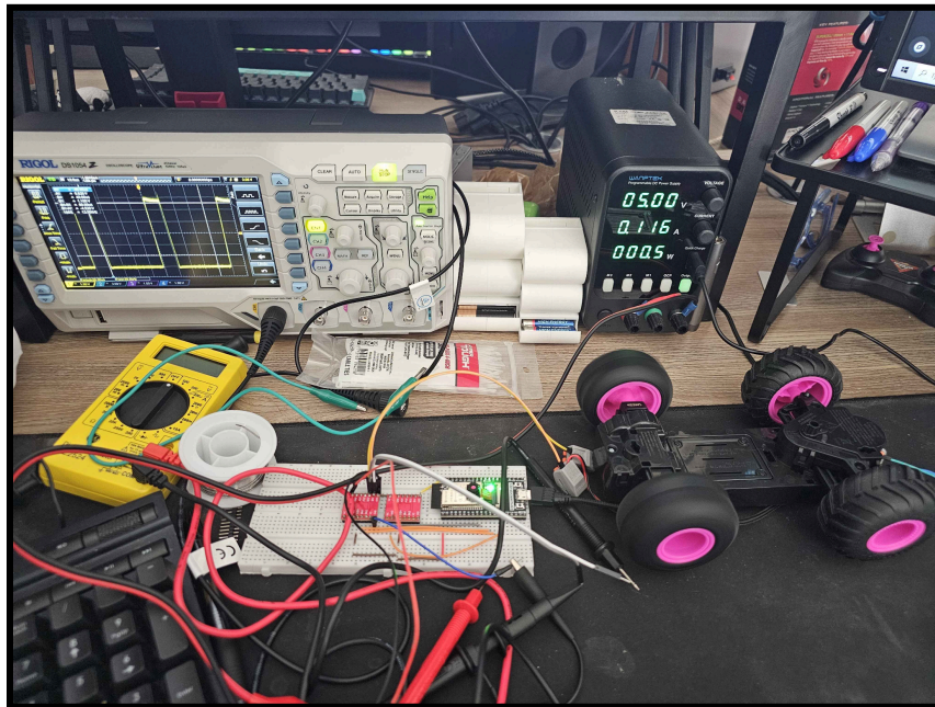
Figure 9.5. Photo from Motor Controls Tests via Motor Driver and ESP32 Connections
